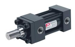
Peninsular hydraulic cylinder, NFPA tie rod, 2in bore, 1-3/8in rod diameter, 2in stroke, double acting, tapped end caps mount.
