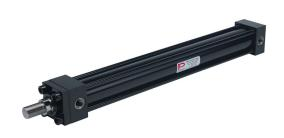
Peninsular hydraulic cylinder, NFPA tie rod, 2in bore, 1-3/8in rod diameter, 20in stroke, double acting, tapped end caps mount.
