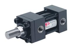
Peninsular hydraulic cylinder, NFPA tie rod, 2in bore, 1-3/8in rod diameter, 1in stroke, double acting, tapped end caps mount.
