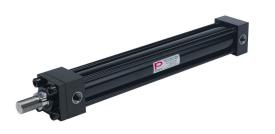
Peninsular hydraulic cylinder, NFPA tie rod, 2in bore, 1-3/8in rod diameter, 16in stroke, double acting, tapped end caps mount.
