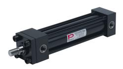
Peninsular hydraulic cylinder, NFPA tie rod, 2in bore, 1in rod diameter, 8in stroke, double acting, tapped end caps mount.
