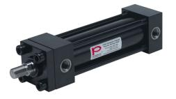
Peninsular hydraulic cylinder, NFPA tie rod, 2in bore, 1in rod diameter, 6in stroke, double acting, tapped end caps mount.
