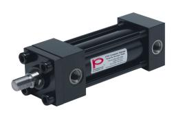
Peninsular hydraulic cylinder, NFPA tie rod, 2in bore, 1in rod diameter, 4in stroke, double acting, tapped end caps mount.
