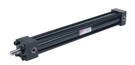
Peninsular hydraulic cylinder, NFPA tie rod, 2in bore, 1in rod diameter, 20in stroke, double acting, tapped end caps mount.
