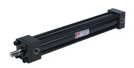
Peninsular hydraulic cylinder, NFPA tie rod, 2in bore, 1in rod diameter, 16in stroke, double acting, tapped end caps mount.
