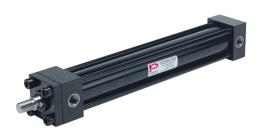
Peninsular hydraulic cylinder, NFPA tie rod, 2in bore, 1in rod diameter, 14in stroke, double acting, tapped end caps mount.
