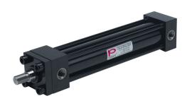
Peninsular hydraulic cylinder, NFPA tie rod, 2in bore, 1in rod diameter, 10in stroke, double acting, tapped end caps mount.
