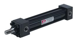
Peninsular hydraulic cylinder, NFPA tie rod, 1-1/2in bore, 1in rod diameter, 8in stroke, double acting, tapped end caps mount.
