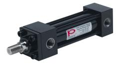
Peninsular hydraulic cylinder, NFPA tie rod, 1-1/2in bore, 1in rod diameter, 4in stroke, double acting, tapped end caps mount.
