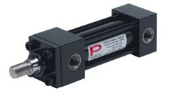
Peninsular hydraulic cylinder, NFPA tie rod, 1-1/2in bore, 1in rod diameter, 3in stroke, double acting, tapped end caps mount.
