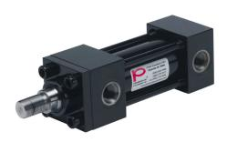
Peninsular hydraulic cylinder, NFPA tie rod, 1-1/2in bore, 1in rod diameter, 2in stroke, double acting, tapped end caps mount.
