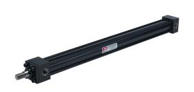
Peninsular hydraulic cylinder, NFPA tie rod, 1-1/2in bore, 1in rod diameter, 24in stroke, double acting, tapped end caps mount.
