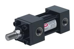
Peninsular hydraulic cylinder, NFPA tie rod, 1-1/2in bore, 1in rod diameter, 1in stroke, double acting, tapped end caps mount.
