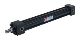
Peninsular hydraulic cylinder, NFPA tie rod, 1-1/2in bore, 1in rod diameter, 14in stroke, double acting, tapped end caps mount.
