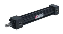
Peninsular hydraulic cylinder, NFPA tie rod, 1-1/2in bore, 1in rod diameter, 10in stroke, double acting, tapped end caps mount.
