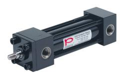
Peninsular hydraulic cylinder, NFPA tie rod, 1-1/2in bore, 5/8in rod diameter, 4in stroke, double acting, tapped end caps mount.
