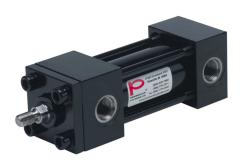
Peninsular hydraulic cylinder, NFPA tie rod, 1-1/2in bore, 5/8in rod diameter, 2in stroke, double acting, tapped end caps mount.
