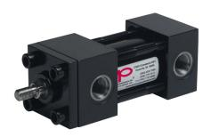
Peninsular hydraulic cylinder, NFPA tie rod, 1-1/2in bore, 5/8in rod diameter, 1in stroke, double acting, tapped end caps mount.
