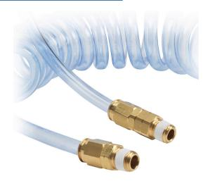
NITRA pneumatic coiled hose, polyurethane, clear blue, 1/4in inside diameter, 0.375in outside diameter, (2) 1/4in male NPT brass fittings (one end fixed, one end swivel), 16ft working length.
