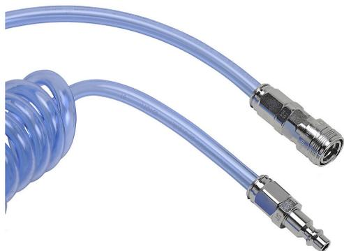
NITRA pneumatic coiled hose, polyurethane, clear blue, 1/4in inside diameter, 0.375in outside diameter, 1/4in chrome plated steel quick-disconnect fittings, 16ft working length.
