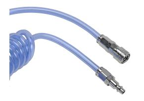
NITRA pneumatic coiled hose, polyurethane, clear blue, 1/4in inside diameter, 0.375in outside diameter, 1/4in chrome plated steel quick-disconnect fittings, 16ft working length.
