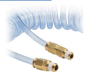
NITRA pneumatic coiled hose, polyurethane, clear blue, 1/4in inside diameter, 0.375in outside diameter, (2) 1/4in male NPT brass fittings (one end fixed, one end swivel), 12ft working length.
