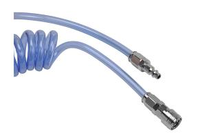
NITRA pneumatic coiled hose, polyurethane, clear blue, 1/4in inside diameter, 0.375in outside diameter, 1/4in chrome plated steel quick-disconnect fittings, 12ft working length.
