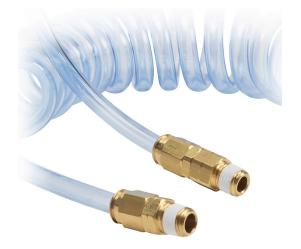
NITRA pneumatic coiled hose, polyurethane, clear blue, 1/4in inside diameter, 0.375in outside diameter, (2) 1/4in male NPT brass fittings (one end fixed, one end swivel), 8ft working length.
