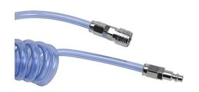
NITRA pneumatic coiled hose, polyurethane, clear blue, 1/4in inside diameter, 0.375in outside diameter, 1/4in chrome plated steel quick-disconnect fittings, 8ft working length.
