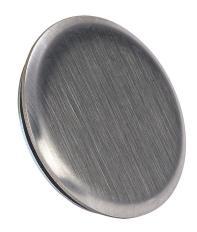
Hammond hole seal, 1-1/4in conduit, 304 stainless steel, #4 brush finish, oil-resistant gasket. For use with stainless steel enclosures.
