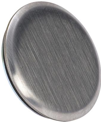
Hammond hole seal, 1-1/4in conduit, 304 stainless steel, #4 brush finish, oil-resistant gasket. For use with stainless steel enclosures.
