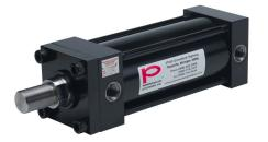
Peninsular hydraulic cylinder, NFPA tie rod, 4in bore, 2in rod diameter, 8in stroke, double acting.
