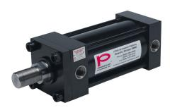
Peninsular hydraulic cylinder, NFPA tie rod, 4in bore, 2in rod diameter, 6in stroke, double acting.
