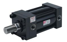
Peninsular hydraulic cylinder, NFPA tie rod, 4in bore, 2in rod diameter, 4in stroke, double acting.
