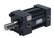
Peninsular hydraulic cylinder, NFPA tie rod, 4in bore, 2in rod diameter, 3in stroke, double acting.
