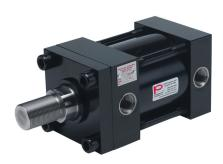
Peninsular hydraulic cylinder, NFPA tie rod, 4in bore, 2in rod diameter, 2in stroke, double acting.
