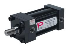
Peninsular hydraulic cylinder, NFPA tie rod, 4in bore, 1-3/4in rod diameter, 5in stroke, double acting.
