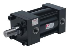
Peninsular hydraulic cylinder, NFPA tie rod, 4in bore, 1-3/4in rod diameter, 3in stroke, double acting.
