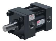
Peninsular hydraulic cylinder, NFPA tie rod, 4in bore, 1-3/4in rod diameter, 1in stroke, double acting.
