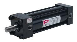
Peninsular hydraulic cylinder, NFPA tie rod, 4in bore, 1-3/4in rod diameter, 10in stroke, double acting.
