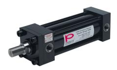
Peninsular hydraulic cylinder, NFPA tie rod, 3-1/4in bore, 1-3/4in rod diameter, 8in stroke, double acting.
