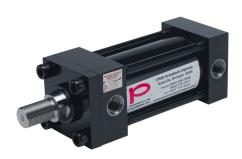
Peninsular hydraulic cylinder, NFPA tie rod, 3-1/4in bore, 1-3/4in rod diameter, 5in stroke, double acting.
