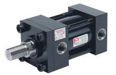
Peninsular hydraulic cylinder, NFPA tie rod, 3-1/4in bore, 1-3/4in rod diameter, 2in stroke, double acting.
