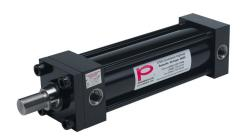
Peninsular hydraulic cylinder, NFPA tie rod, 3-1/4in bore, 1-3/4in rod diameter, 10in stroke, double acting.
