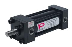
Peninsular hydraulic cylinder, NFPA tie rod, 3-1/4in bore, 1-3/8in rod diameter, 6in stroke, double acting.
