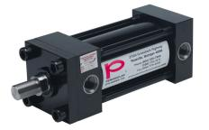
Peninsular hydraulic cylinder, NFPA tie rod, 3-1/4in bore, 1-3/8in rod diameter, 5in stroke, double acting.
