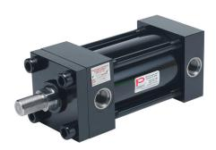
Peninsular hydraulic cylinder, NFPA tie rod, 3-1/4in bore, 1-3/8in rod diameter, 4in stroke, double acting.
