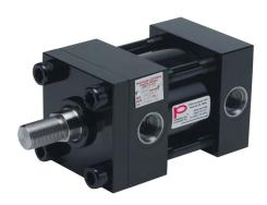
Peninsular hydraulic cylinder, NFPA tie rod, 3-1/4in bore, 1-3/8in rod diameter, 1in stroke, double acting.
