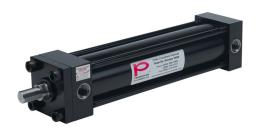
Peninsular hydraulic cylinder, NFPA tie rod, 3-1/4in bore, 1-3/8in rod diameter, 14in stroke, double acting.
