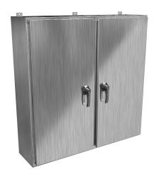
Hammond enclosure, NEMA 3R/4X/12/13, 48 x 48 x 12in (HxWxD), wall mount, 304 stainless steel, #4 brush finish, 2-door, 3-point 316 stainless steel padlocking handle.
