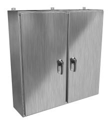
Hammond enclosure, NEMA 3R/4X/12/13, 48 x 48 x 12in (HxWxD), wall mount, 316 stainless steel, #4 brush finish, 2-door, 3-point 316 stainless steel padlocking handle.
