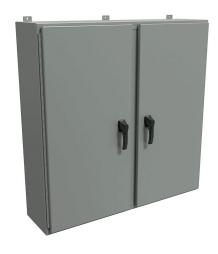
Hammond enclosure, NEMA 3R/4/12, 48 x 48 x 12in (HxWxD), wall mount, carbon steel, ANSI 61 gray, powder coat finish, 2-door, 3-point padlocking handle.
